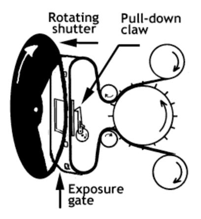
Shutter speed to shutter angles at 24 fps the math is (24 x 360) / Time Fraction
