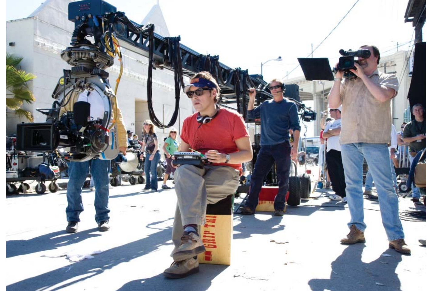
Super Technocrane with stabilized head. Director Joe Wright seated; dolly grip John Mang in dark blue shirt; camera operator Mitch Dubin at far right in background.
