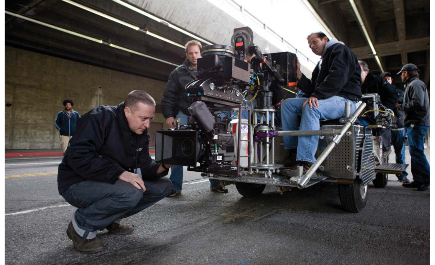
Seamus McGarvey demos setup with camera car, crane arm, inverted Panahead and HotGears. 1 st AC Bill Coe (in jeans) is on the car.
