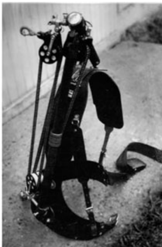
The crane acquired a Kenyon gyro and was supported by a bungee cord running through yacht pulleys.
