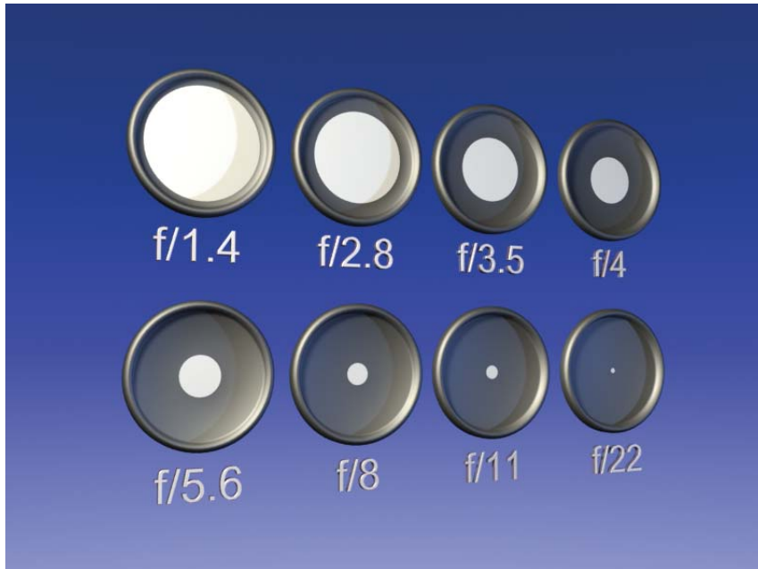
2.1 An aperture on a camera lens works like the iris of your eye, opening and closing to allow more or less light into the camera.
