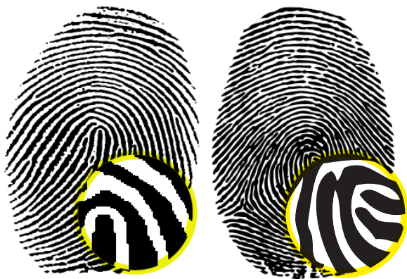
Figure 5. The fingerprint on the left is a raster image, the fingerprint on the right is a vector image.
